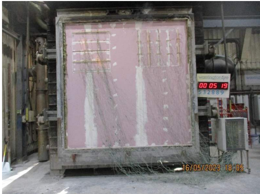
The unexposed face after a test duration of 5 minutes 19 seconds
