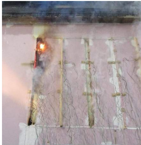
The unexposed face showing flaming on specimen B1
