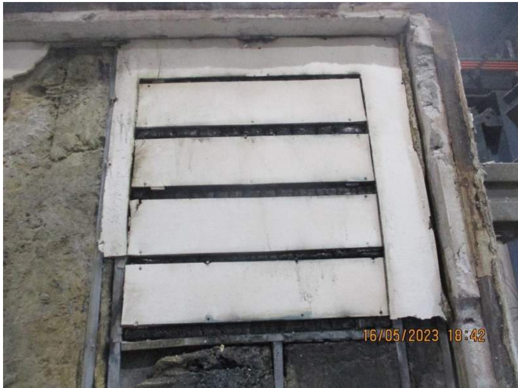
The exposed face after a test duration of specimens Ax after the completion of the test
