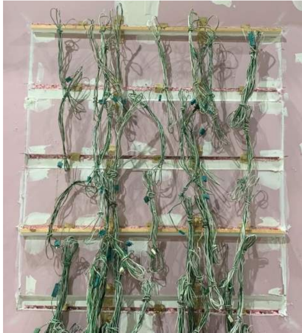
The unexposed face of specimens Ax prior to testing
