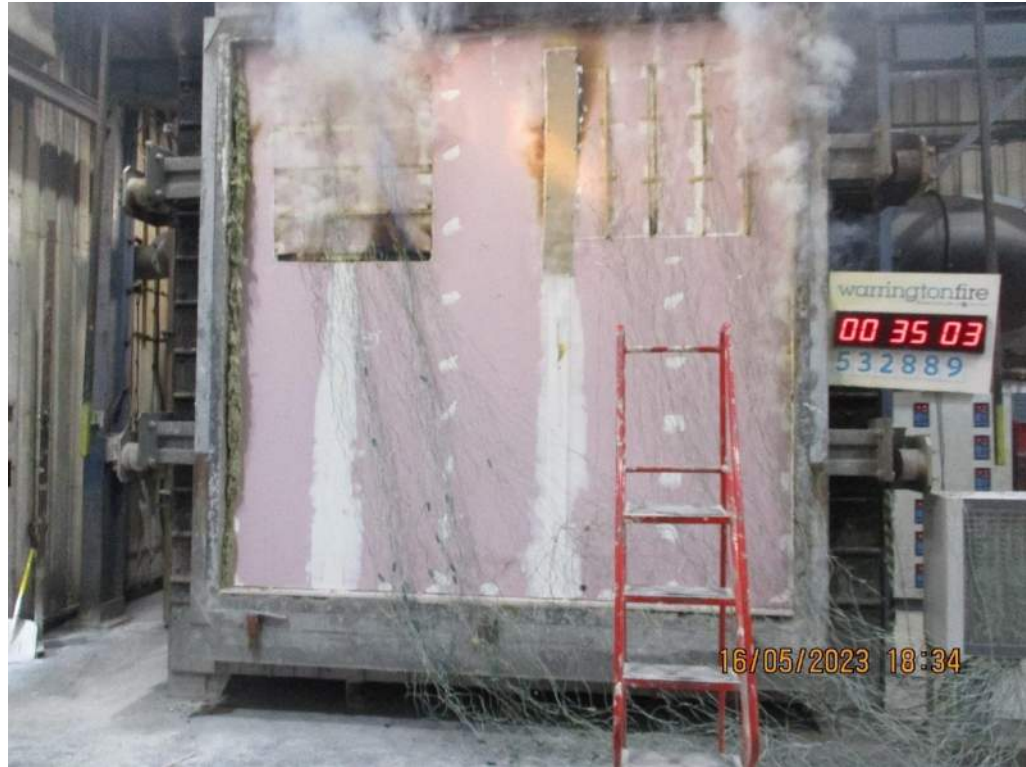
The unexposed face after a test duration of 35 minutes 3 seconds
