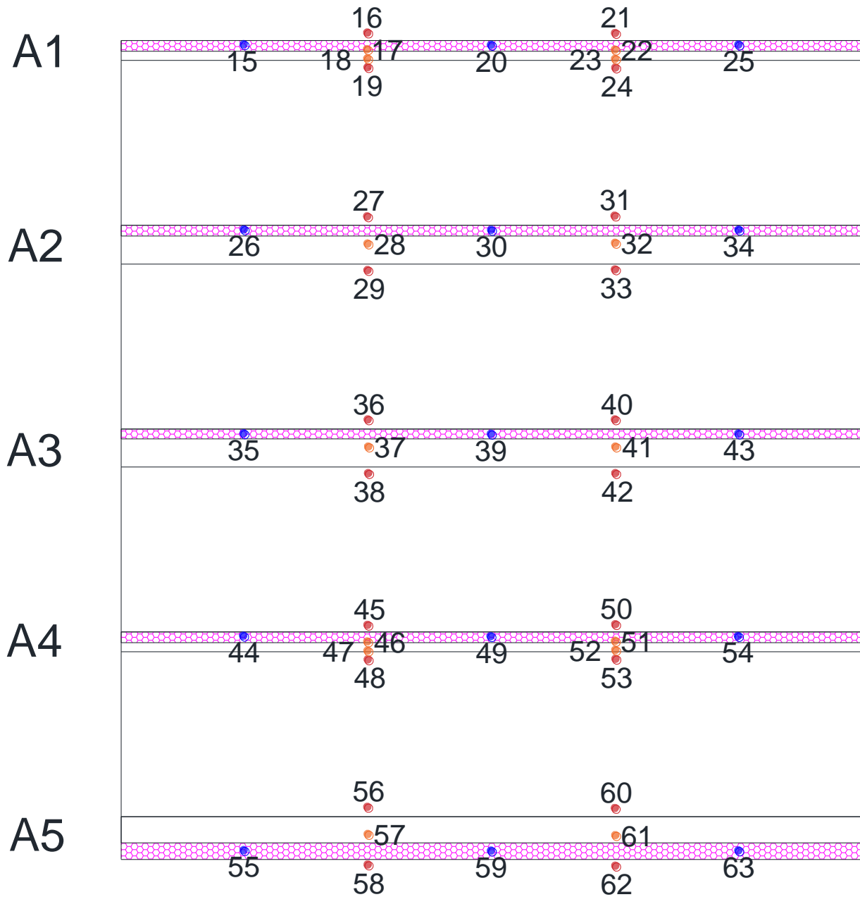
Figure 2 – Unexposed face elevation of the specimens A1 to A5 with thermocouple locations
