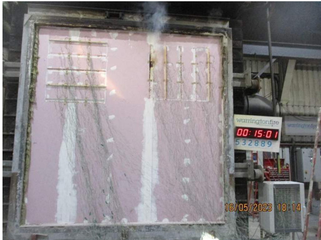
The unexposed face after a test duration of 15 minutes 1 second
