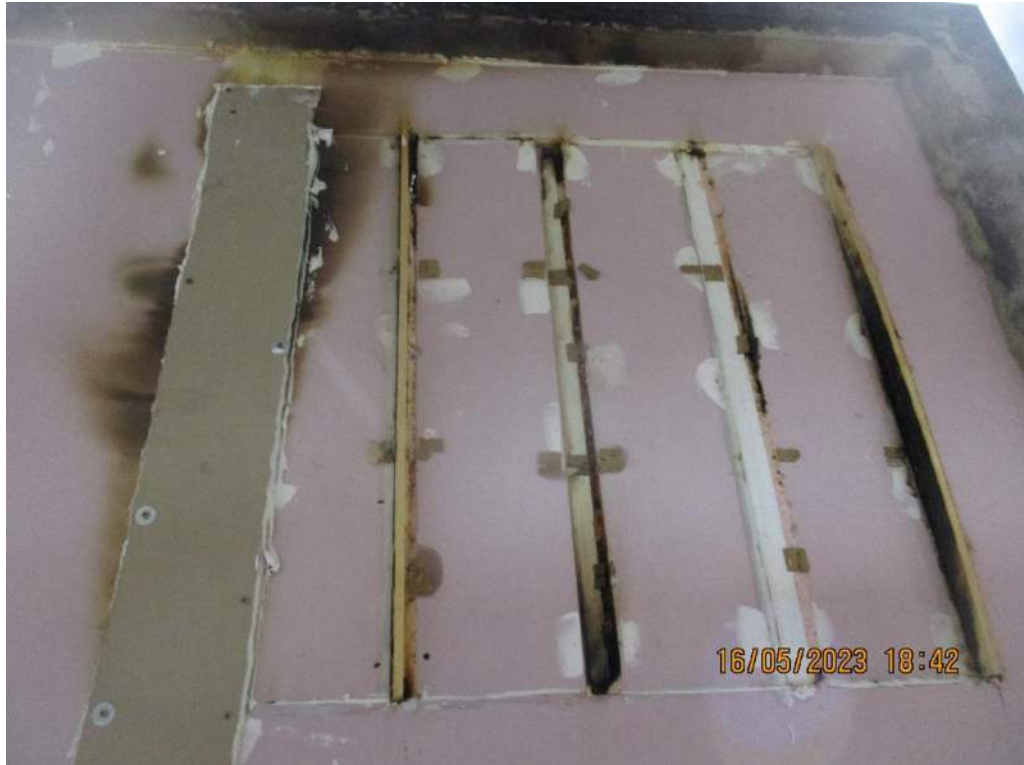
The unexposed face after a test duration of specimens Bx after the completion of the test
