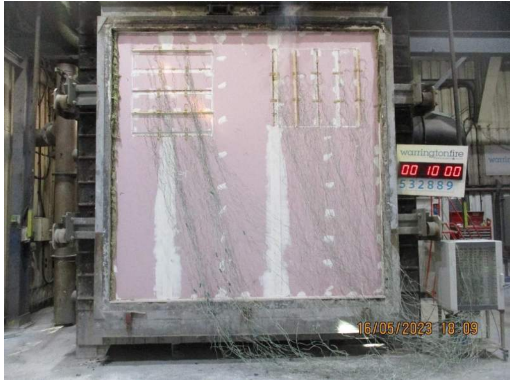
The unexposed face after a test duration of 10 minutes
