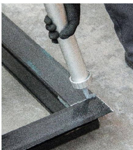
07 Apply the adhesive to all connection joints
